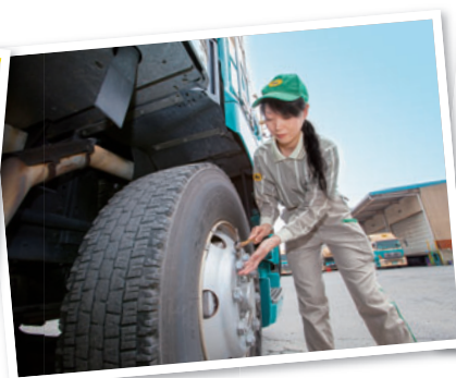
Inspection of wheel bolts prior to leaving
