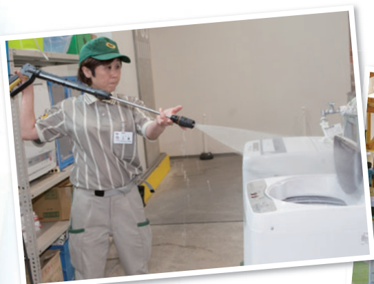
Cleaning the outside of a washing machine with a high pressure cleaner
