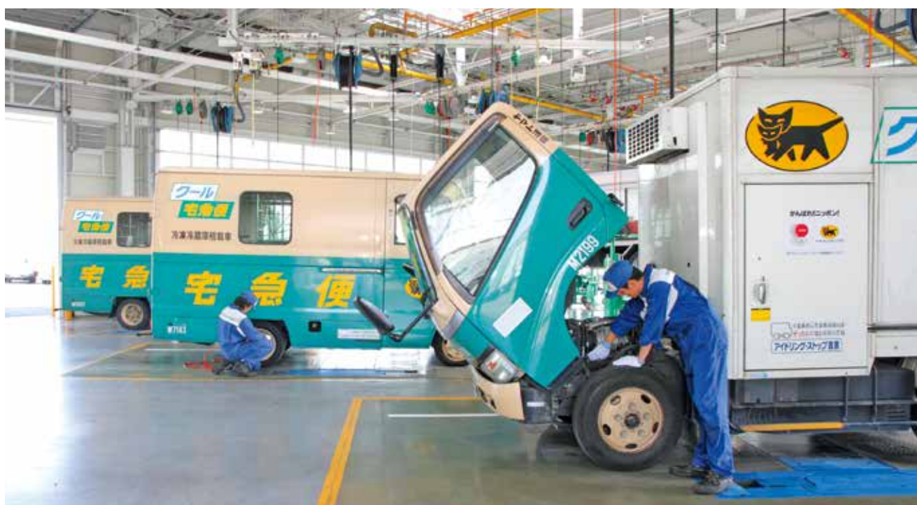
Superworks Saitama Plant: One of the features of Superworks is a “one-direction” traffic line that enables mechanics to perform maintenance on a vehicle without reversing it.
