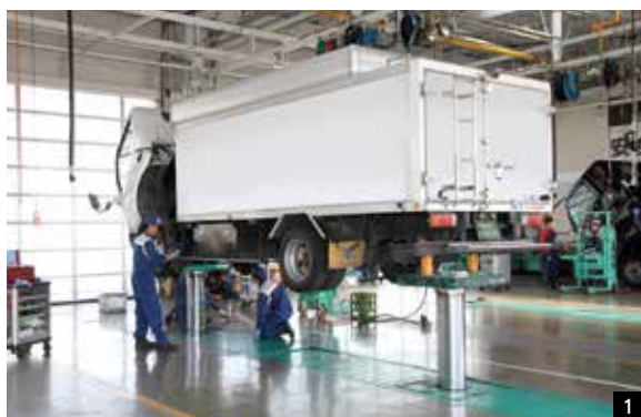
1 Twin Power Lift: As the rear lifting arm moves according to the size of a vehicle body, it can handle various types of vehicles from light vehicles and heavy trucks.
