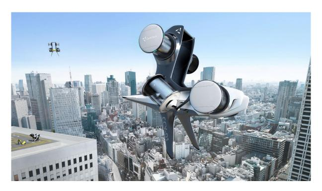
CycloRotors are based on the same principle as the Voith-Schneider-Propeller, successfully applied for decades for highly agile and stable ships in the maritime industry. The compact design and direct and instant control of magnitude and direction of thrust offer a natural, stable transition from hover to forward flight and superior maneuverability. The unique characteristics of CycloRotors give vehicle manufacturers unprecedented freedom in designing and operating aircraft and drones.
