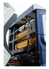
⟨Fuel Cell System and High-Pressure Hydrogen Tanks
