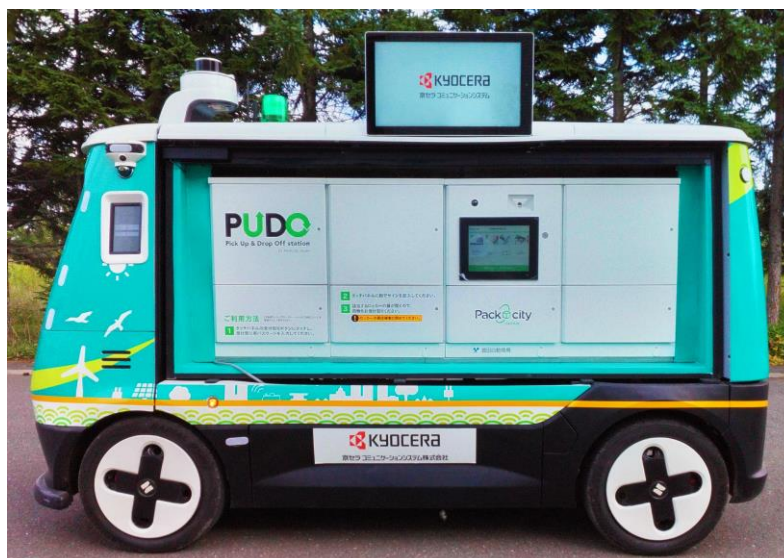
Medium-speed, medium-sized unmanned automated delivery robot
